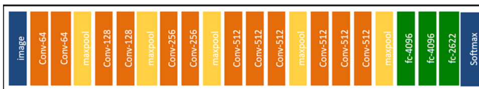
Fig. 9: VGG-Face model exploits in its 22 layers
