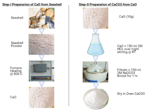
Fig. 2: Synthesis of bio-CaCO_3 via a two-step process namely calcinations and chemical treatment. [15]
