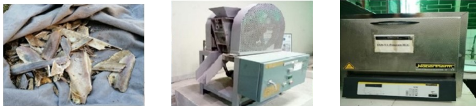
Fig. 3: (a) Bones, (b) crushing of bones using crusher, (c) pyrolysis of bones
