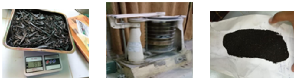
Fig. 4: (a) Bone char, (b) sieving process of bone char, (c) after Sieving bone char
