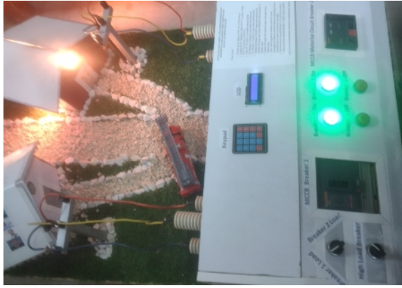
Fig. 5: Breaker 1 and breaker 2 ON Condition.
