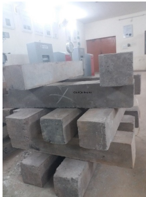
Fig. 4: 0% RAC beams after 6-hour fire
