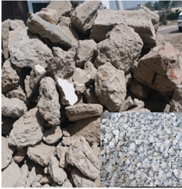
Fig. 3: Old concrete blocks and aggregates
