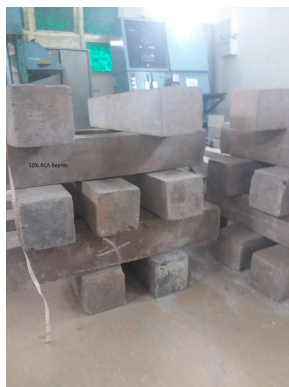
Fig. 5: 50% RAC Beam after 6-hour fire
