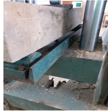
Fig. 6: Testing of beam UTM
