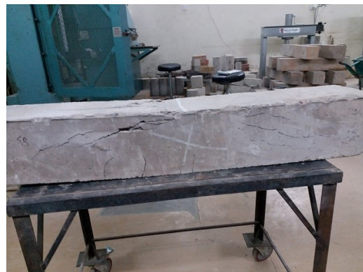
Fig. 11: Cracking in 0% RCA beam
