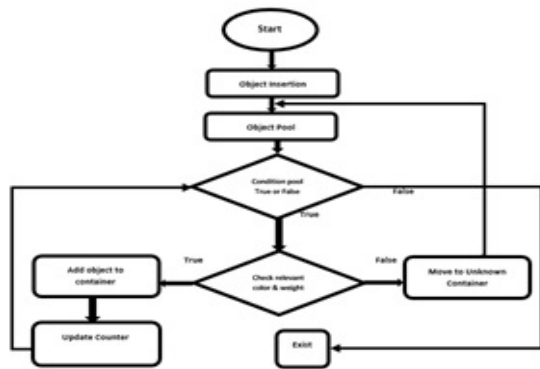
Fig. 1: Logical Architecture of ISOIT
