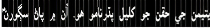
Fig. 7: Vertical segmentation of a Sindhi text line showing ligature boundaries. Each vertical white line represents a successfully identified ligature break extracted through projection profiling.
