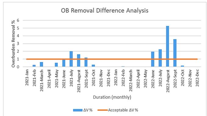
Fig. 5: Comparison between V and acceptable V
