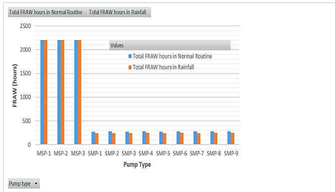
Fig. 6: Comparison between FRAW hours for dewatering pumps
