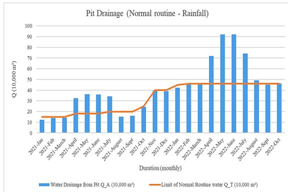
Fig. 7: Pit Dewatering comparison (Normal-Routine – Rainfall)
