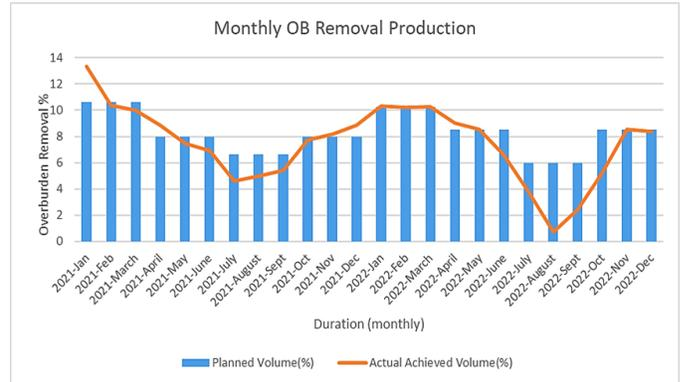
Fig. 4: Comparison between planned (VP) and actual achieved (VA) volumes of OB removed
