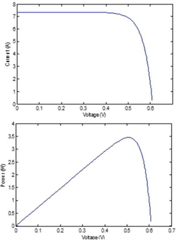
Fig. 4: PV cell characteristics; I-V and P-V (MATLAB ®)
