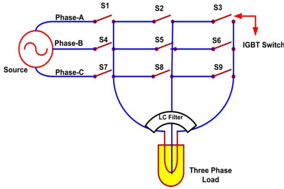
Fig. 1: Simplified 3×3 Matrix Converter
