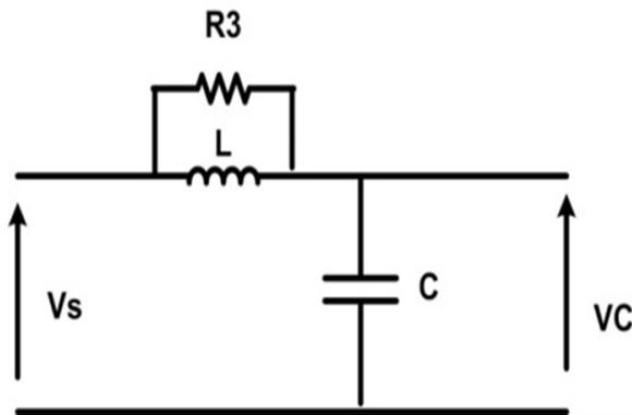
Fig. 11: Resistor connected in parallel to the inductor
