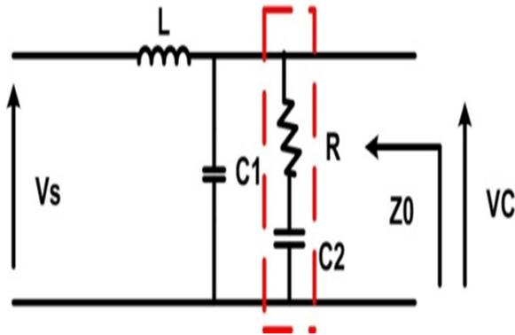
Fig. 7: The improved LC filter
