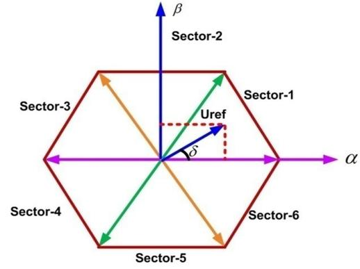
Fig. 3: Output voltage space vectors
