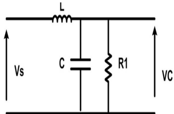
Fig. 9: Resistor connected in parallel to the Capacitor
