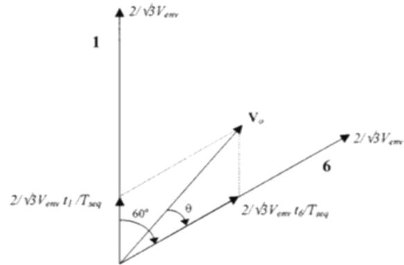
Fig. 4: Output voltage space vectors synthesis
