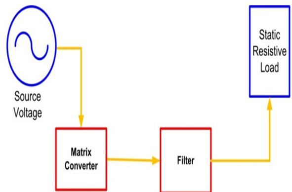
Fig. 14: Block diagram of Three Phase AC to AC Matrix Converter driving Static Resistive Load
