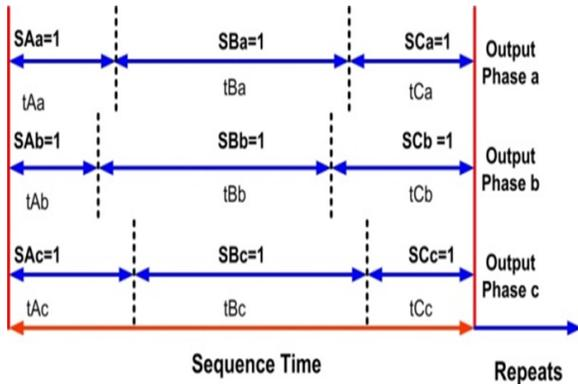
Fig. 2: Common usage of the switching arrangement
