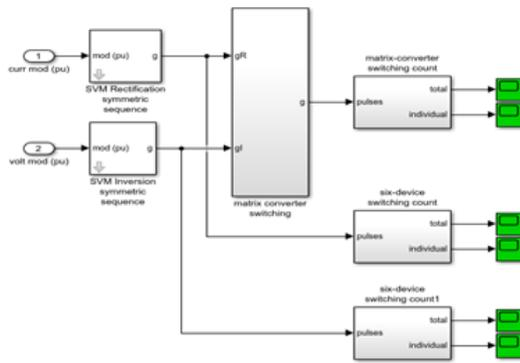
Fig. 15: Simulation Model of Three Phase Matrix Converter
