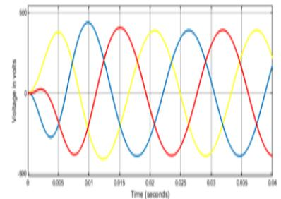
(a) Output Voltage of Three phase Matrix Converter driving Static Load with LC filter
