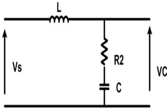
Fig. 10: Resistor connected in series to the capacitor
