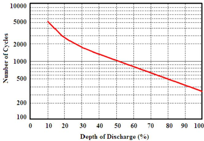
Fig. 3: Battery life cycle versus depth of discharge.
