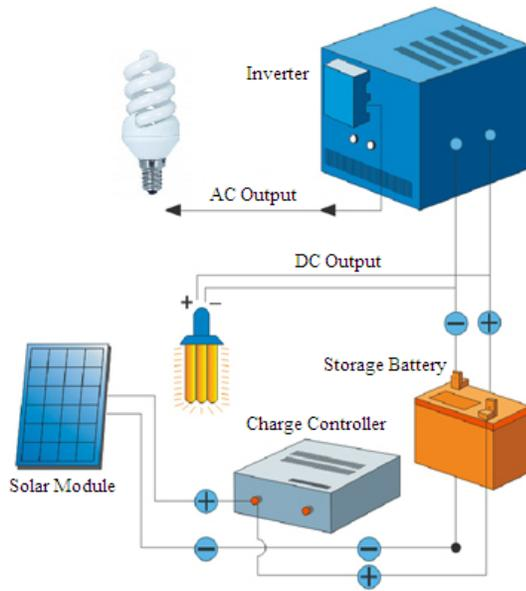
Fig. 1: Components of solar home System .
