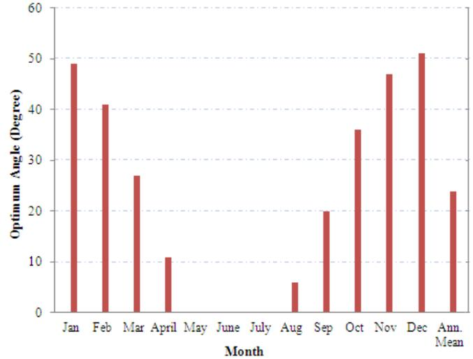
Fig. 6: Monthly average optimized angle for installation of PV panels at Chachro, Thar.
