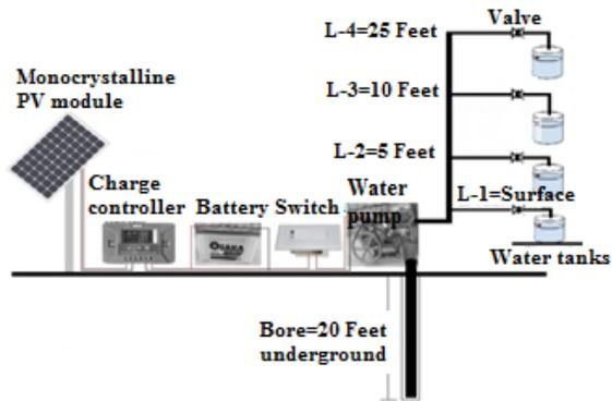
Fig. 1: Schematic diagram of installed water pumping system
