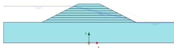
Fig. 6: Pattern of phreatic level in road embankment adopted for 7 m high flood water
