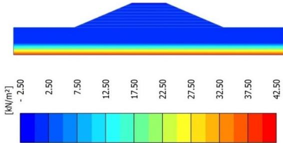
Fig. 10: Pore pressures in the road embankment after end of construction
