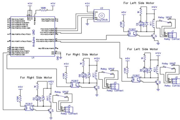
Fig. 6: Schematic diagram of the driving mechanism
