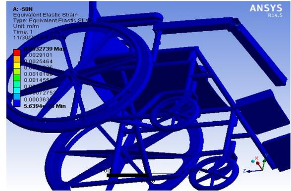
Fig. 12: Simulated results of equivalent elastic strain over 50N of force
