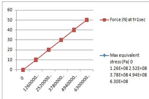
Fig. 11: Relation between force and maximum equivalent stress
