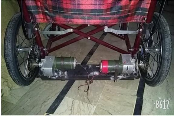
Fig. 4: Manual wheelchair with motor assemble
