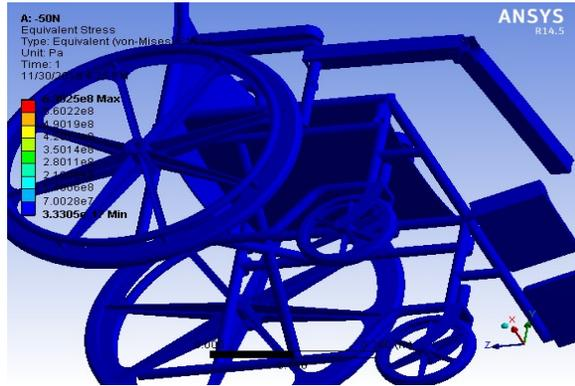
Fig. 10: Simulated results of equivalent stress over 50N of force
