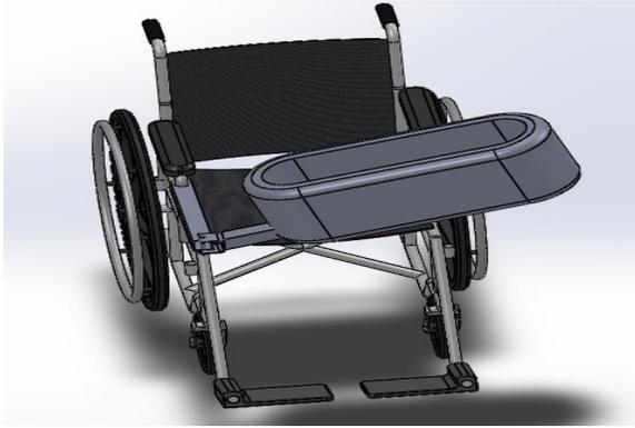
Fig. 1: Solid works model for the carrier attachment
