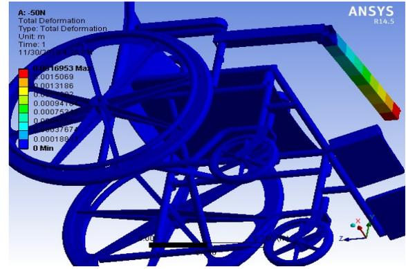
Fig. 8: Simulated results of total deformation over 50N of force
