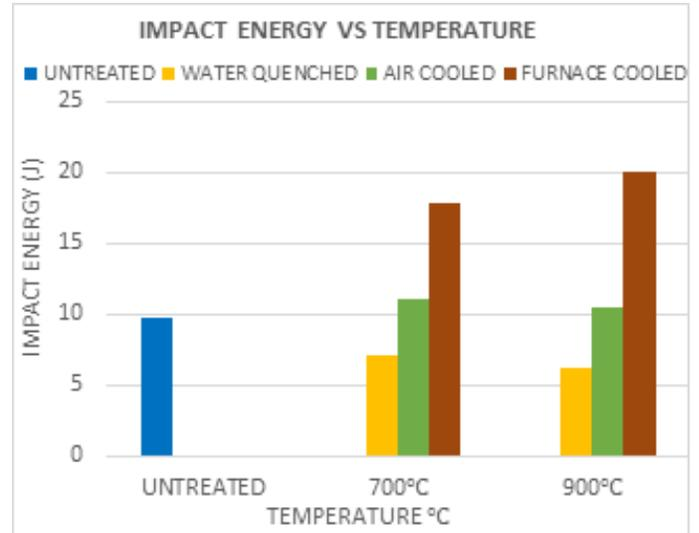
Fig. 2: Impact energy at 700°C and 900°C with different cooling conditions (after 90 min austenitization)
