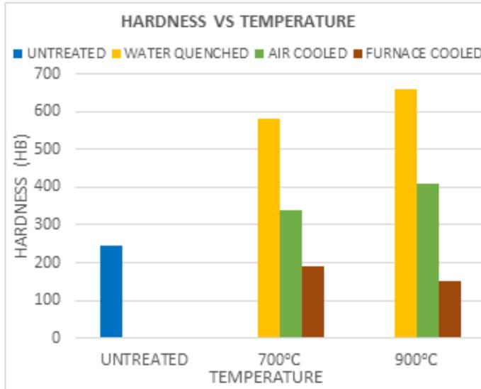
Fig. 3: Hardness value at 700°C and 900°C with different cooling conditions (after 90 min austenitization.)
