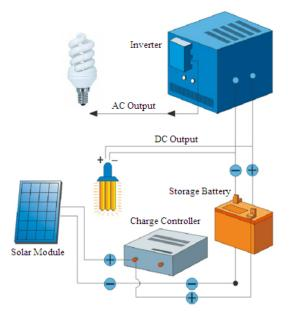
Fig. 1: Components of solar home System.
