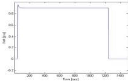
Fig. 8 Battery current at full charging rate
