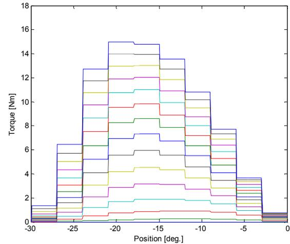
Figure 3.2 Torque versus rotor position [under linear]
