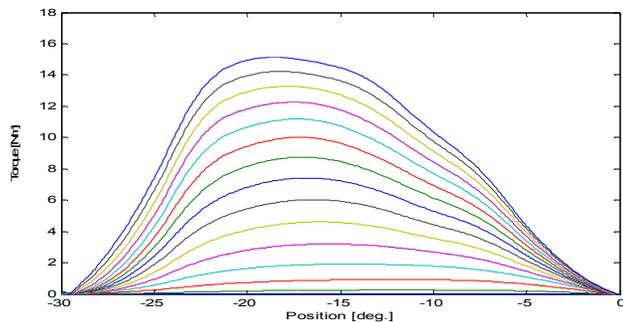
Figure 3.1 Torque versus rotor position [under spline]
