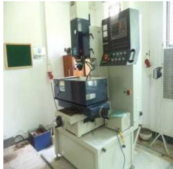
Fig.2 Electrical Discharge Machine (EDM) Die Sinker
