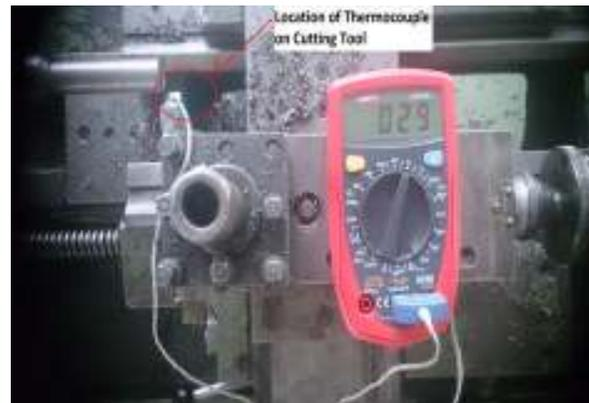
Fig.3 Thermocouple arrangements on tool
