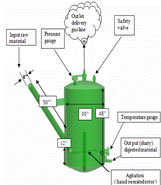
Fig 1: Anaerobic Digester (Batch-Type)
