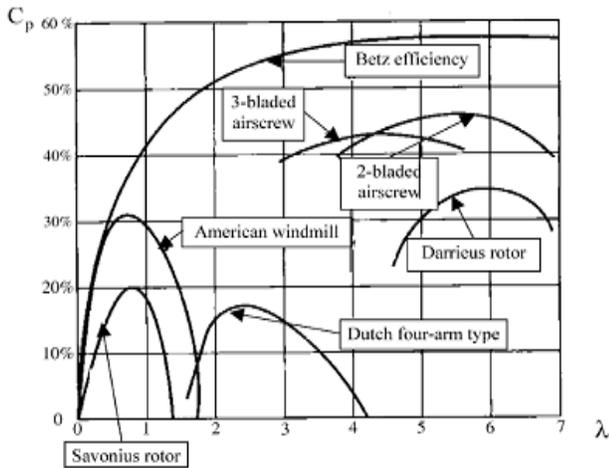
Fig. 4: Characteristic curves of many conventional wind machines
