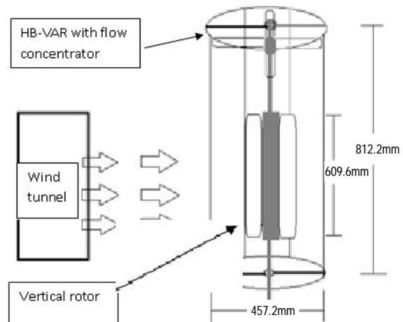
Fig 1: Test Setup Drawings
