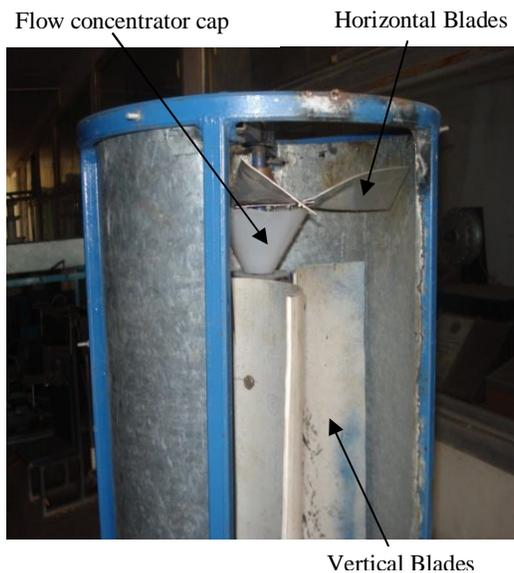
Fig 3: Test setup
