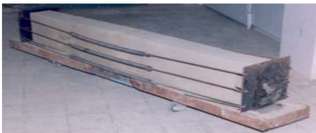
Figure 3: Photograph of the system used to avoid the cracking in the clay beams due to shrinkage.
