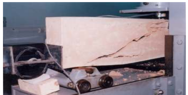
Fig. 10: Photographs showing the cracks after testing the beam
