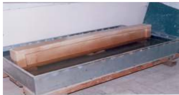
Figure 4: The tube to cure the baked clay beam after grouting
