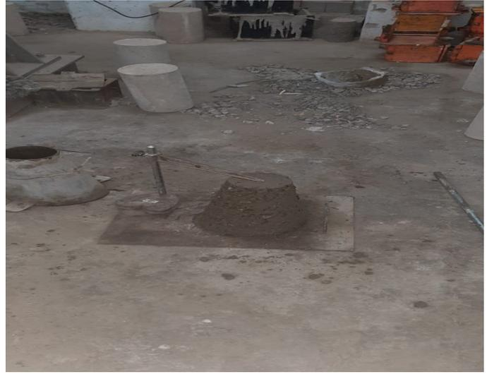
Fig. 4: Slump test
