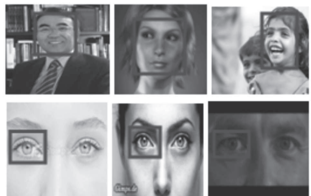
Fig. 5: Face and eye detection using the strong classifiers
