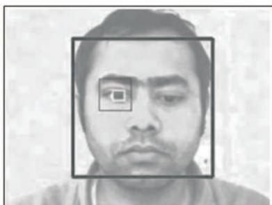
Figure. 6: Iris tracking after face and eye detection
